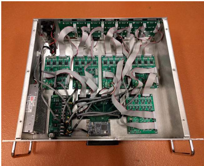
FIG. 1. Low Voltage chassis with board Q0131 in the lower right corner.
